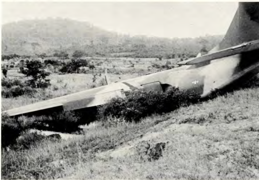
Aircraft that crash land near back country airstrips pose interesting recovery problems for AFLC's RAM teams. Whenever possible, the aircraft are temporarily repaired and flown to a major U. S. Air Base for Depot level maintenance.
