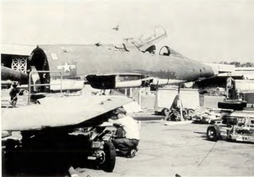
When crash or battle damage is too severe to be repaired at overseas locations, RAM teams disassemble the aircraft piece by piece and package the parts for shipment to an AFLC depot in the CONUS.
