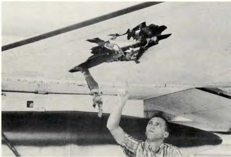
An AFLC civilian mechanic points to battle damage in the outer wing of an F-4 Phantom in Southeast Asia. Repair of such damage is often beyond the capability of bases in Vietnam and RAM teams are called in to assist.
