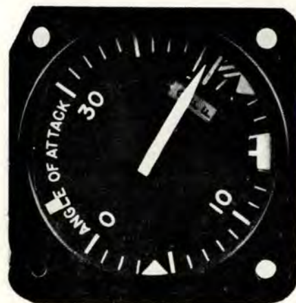
F-4 angle of attack indicator works in conjunction with approach indexer lights; both have been widely accepted by pilots.
